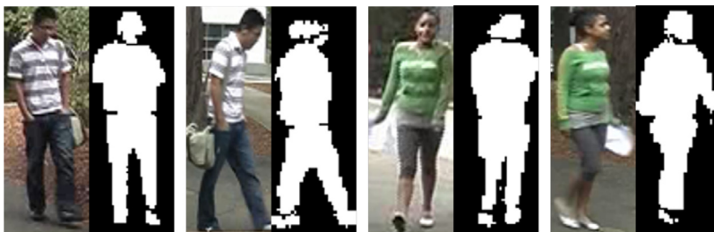
Fig. 3. Sample segmentation results using the method in [43] to separate the foreground subject from the background. The appearance features are extracted from the foreground to mitigate the impact by the cluttered background.
